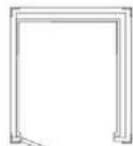
Manually operated door
